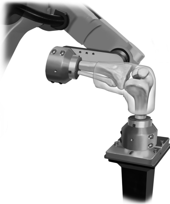
Figure 1. Schematic representation of the robotic setup with the inverted knee mounted in the testing system.
